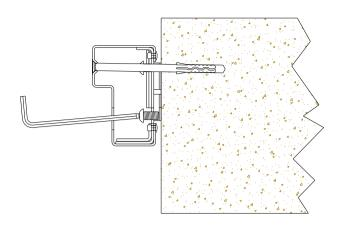
**9.** Open the door fully, then tighten the frame adjusters in the reveals. Using the 5mm Allen key, tighten the frame adjusters until the ends of the spreader plates are flat against the wall.
