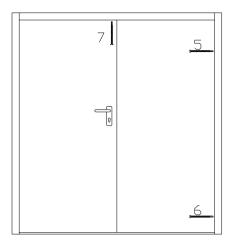
**8.** Close the active leaf again, then fit the last 2 fixings into face 5 of the fixed leaf jamb and 1 into the head.
