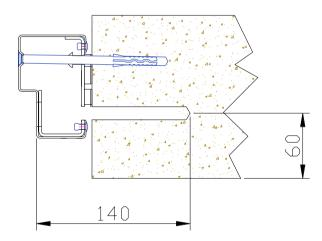
10. Drill through the access holes in the reveals with a 12mm masonry bit, to a depth of 140mm.
